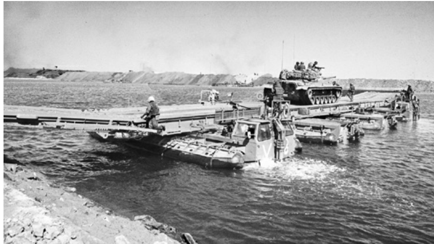
Amphibious bridging tugs put the first Israeli tanks across (illustration credit ill.30)
