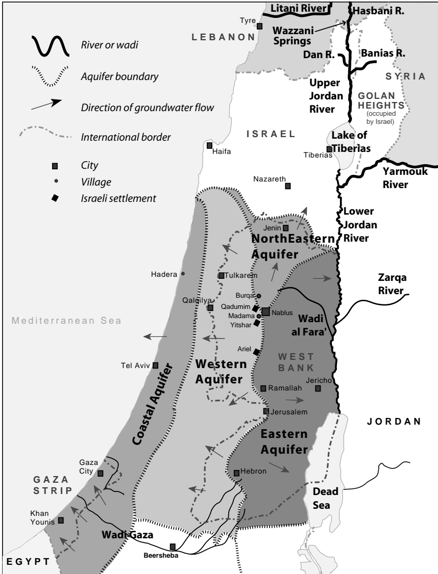
Figure 3.1 Transboundary surface water and groundwater resources of Palestine and Israel: Jordan River System and four aquifers.
